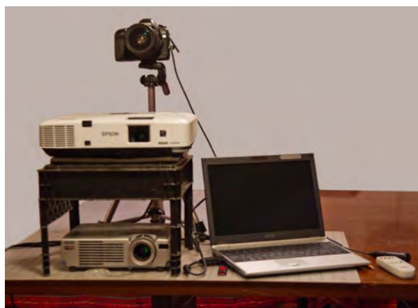
Figure 1. Test set-up with two projectors, laptop computer, and camera..
